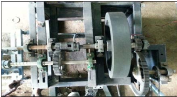
Figure 1.3: Mechanical power transmission unit.
