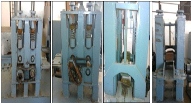
Figure 1.4: Different views of bamboo sliver cutting unit.
