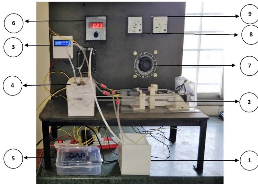
Figure 13.2: Typical experimental setup where Coolant tank (1), Syringe pump (2), Digital differential pressure transducer (3), Microchannel test section (4), Rectangular cartridge heaters (5), Thermostat (6), Data Acquisition system (7), Computer (8), Radiator (9), Digital temperature indicator (10) and Glass wool.
