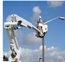
Preventing electrocutions and falls with 3-dimensional roller arms (12)
