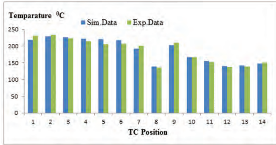
Figure 3.5: Simulation and experimental results of temperature distributions.
