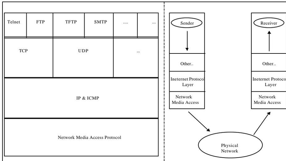
Figure 2-3: Typical Sender/Receiver utilizing TCP/IP (Source: adapted from Comer p.139)
