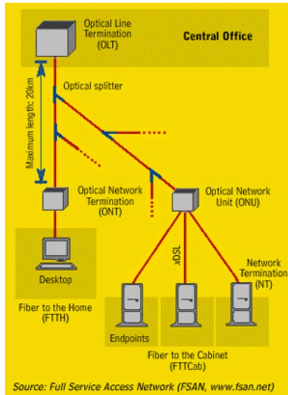
**Nothing but Glass.** Between the Optical Line Terminal (OLT) at the Central Office (CO) and up to 32 Optical Network Units (ONUs), low-cost passive optical splitters distribute optical signals without requiring electricity.
